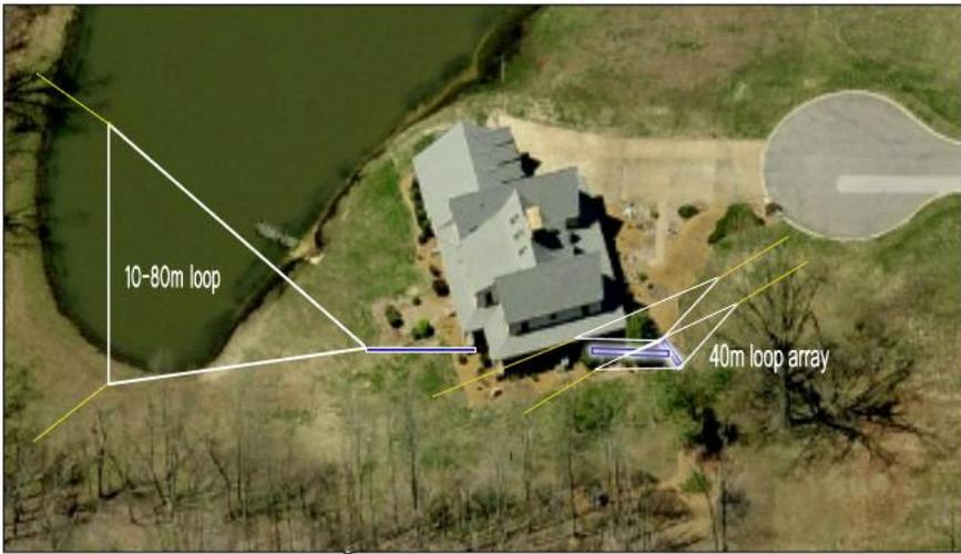
Decided to position the new array in the location shown above. I decided to use four suitable lengths of black dacron halyard to suspend the top two legs of the array between trees at a height of about 50 ft. The relative position of the 300 ohm feed line and relay system is shown in blue. Note that the array faces nearly West - East.
